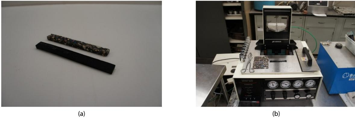
Fig. 1. BBR Binder Mixture Test Specimen (a) and Testing Equipment Setup (b)
