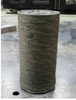
(a) Cylinder for Compressive Strength
